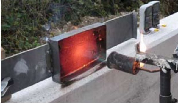
Aerogel and firewall section during tests:
