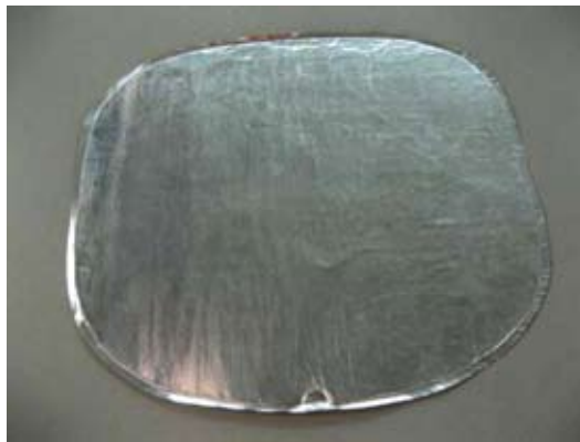
Thin, light weight encapsulated 6 mm Pyrogel with self-adhesive cold side
