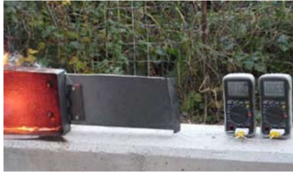
Cold side temperatures (ambient temperature: 10°C):
