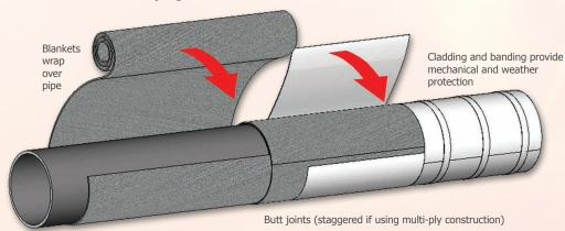
Installation of flexible Pyrogel XT blankets is fast and intuitive.
