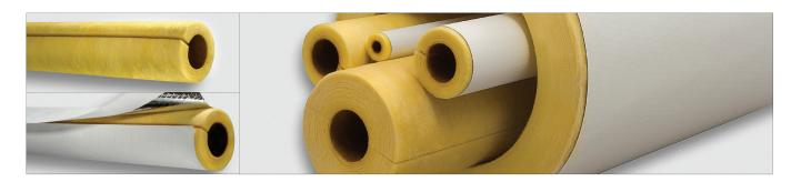
**ALLEY-K**<sup>TM</sup> is a preformed pipe insulation composed of high quality glass fibres, bonded together with a thermosetting resin. The 36" pipe sections are available with or without the all service jacket (ASJ). Our all service vapour retarder jacket (ASJ) reinforced with glass fibres comes with a factory applied pressure sensitive self-sealing lap closure system (SSL). Butt strips are also supplied.
