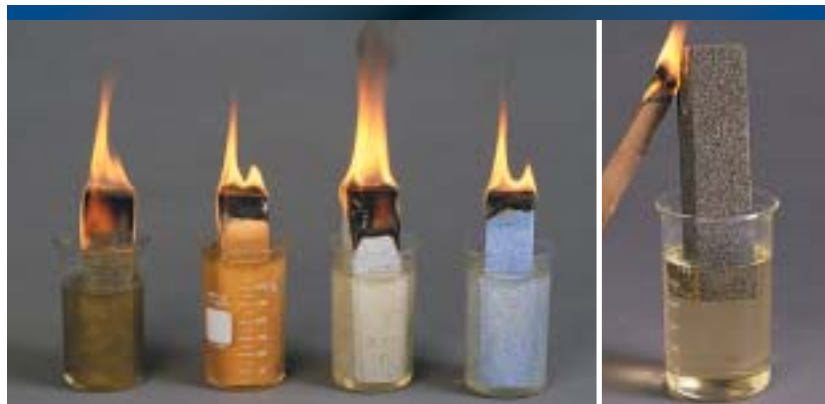
FOAMGLAS® insulation (above) remains non-wicking and non-burning while mineral wool, calcium silicate and two brands of perlite sustain flames from wicking of oil.
