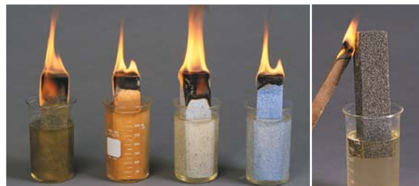
FOAMGLAS® insulation (above) remains non-wicking and non-burning while mineral wool, calcium silicate and two brands of perlite sustain flames from wicking or oil.
