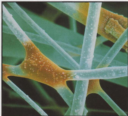
A magnified view of ROXUL mineral wool shows its interlocking structure and the water repellent coating. These fibres are approximately 1/15th the size of a human hair.
