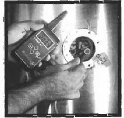
A UT METER IS USED TO MAKE PROPER INSPECTION
