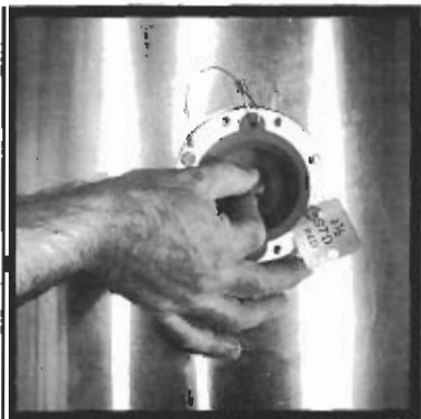
PULL CENTER NIPPLE TO BREAK SEAL
