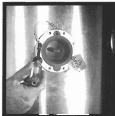
INSTALL 2 SELF STARTING SCREWS ACROSS FROM EACH OTHER, ONE FOR A SAFETY LINE AND THE OTHER FOR HOLDING AN I.D. TAG
