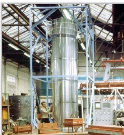
Representative insulation test to ascertain thermal performance at ranging temperatures.
