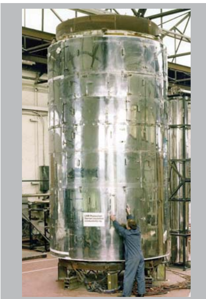
Representative insulation test to ascertain thermal performance at ranging temperatures.
